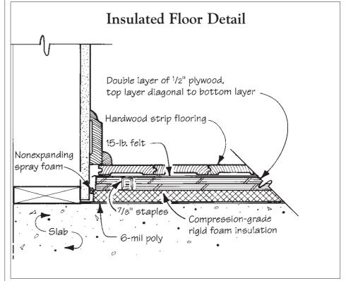
This detail shows one way to lay an insulated wood floor over an uninsulated concrete slab, using 1-inch (R-5) extruded polystyrene. More foam can be added for more insulating value. To prevent movement and possible floor squeaks, it's important to keep the foam flat and well supported.
