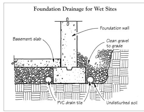
In areas with a high seasonal water table, a foundation should have both interior and exterior perimeter drains. Run the drains to daylight or to a sump pump connected to a storm drain.
