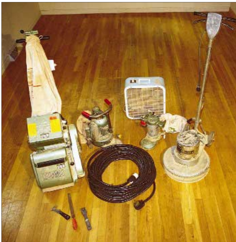
Figure 1. Tools of the flooring trade. You won't find a drum sander like this one (at left in photo) in a rental shop — the professional model weighs more, costs more, and produces better results. The author uses two sizes of edge sanders for greater flexibility in tight spots. Ordinary hand scrapers (bottom left in photo) go where the edgers won't. Screening with the buffer/polisher removes sanding marks and buffs between finish coats. The heavy extension cord allows the author to get 240-volt power from the home's range or dryer outlet. When weather permits, the window fan reduces dust.
