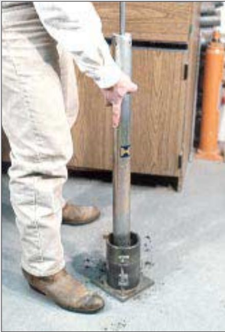
Figure A. In the standard Proctor test, a soil sample is mixed with water, then layered into a sturdy metal cylinder (left). A 5½-pound weight is dropped 25 times from a height of 12-inches to compact the sample. To get wet density, the volume occupied by the compacted sample is divided into its weight (above). After the sample is dried in an oven, the same calculation yields dry density.
