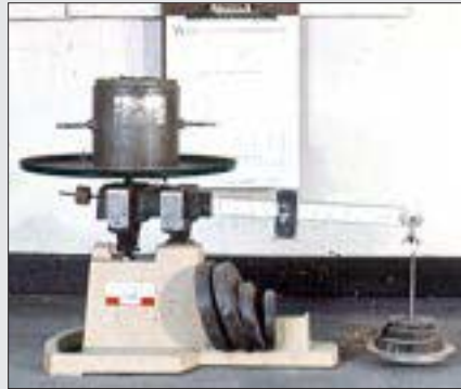
Figure A. In the standard Proctor test, a soil sample is mixed with water, then layered into a sturdy metal cylinder (left). A 5½-pound weight is dropped 25 times from a height of 12-inches to compact the sample. To get wet density, the volume occupied by the compacted sample is divided into its weight (above). After the sample is dried in an oven, the same calculation yields dry density.
