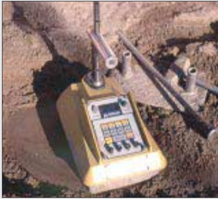
Figure C. To test soil density on site, field engineers use a nuclear gauge. With the keypad, the engineer can do the calculations for an immediate readout of percent compaction.
