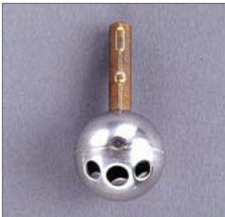
Figure M. Some inexpensive single-lever faucets use a plastic ball to control water flow. This should be replaced with a stainless steel ball like the one shown here.
