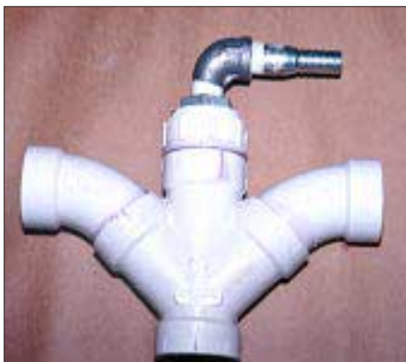
Figure D. For connecting a dishwasher, a double-Y fitting with a galvanized reducer in the center hub works well.
