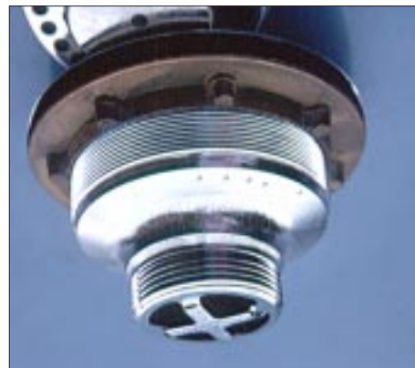
Figure B. The author likes the Kohler Duostrainer for kitchen sinks — its cut threads are less likely to leak than the rolled threads on cheaper strainers.
