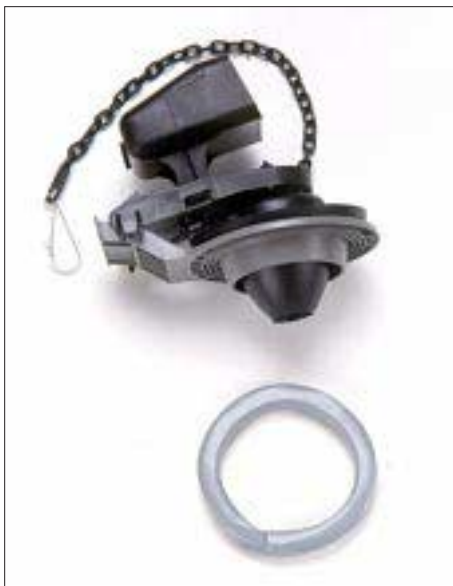
Figure H. This flapper replacement kit comes with a putty ring for cushioning jagged edges in the outlet of the toilet tank, ensuring a good seal.
