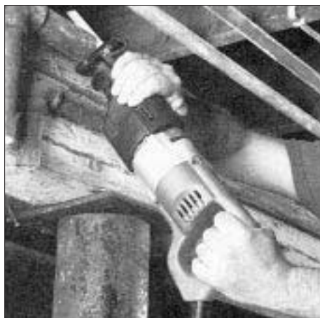
The Super Sawzall features dial-in speed control, and an adjustable shoe for better control when cutting heavy material, such as these iron pipes.
