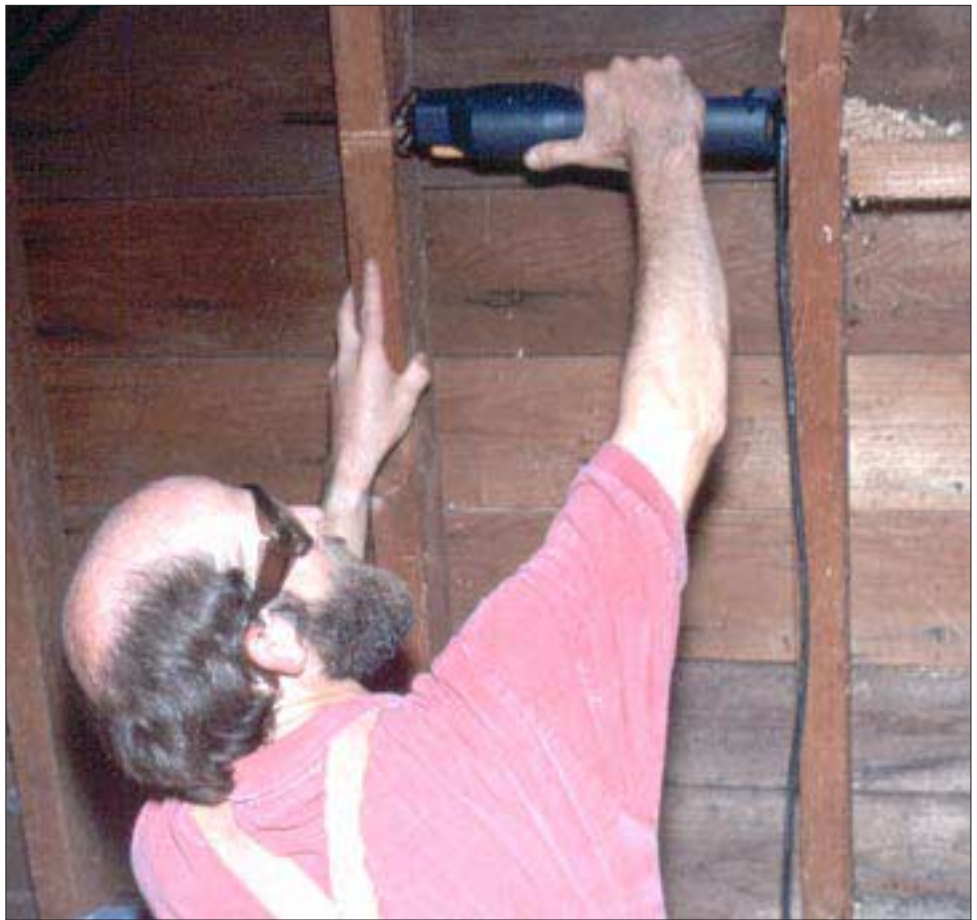
Though it's smaller and less powerful than a reciprocating saw, the new Bosch B4050 in-line jigsaw will fit into a joist or stud bay and can be operated with one hand.
