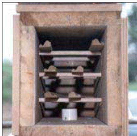
E. Inside the steam box, 1/2-inch dowels support the moldings for steaming.
