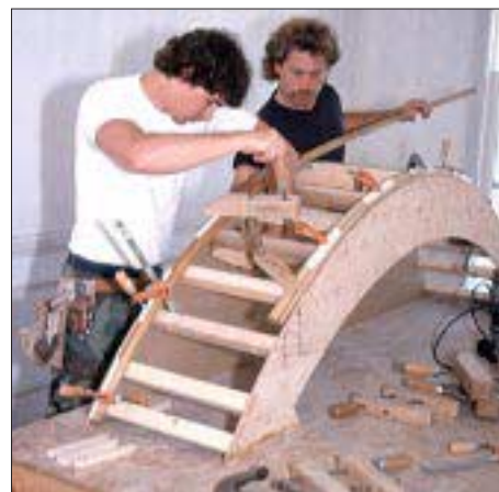
F. After steaming, the long moldings are clamped on a radiused form to dry.
