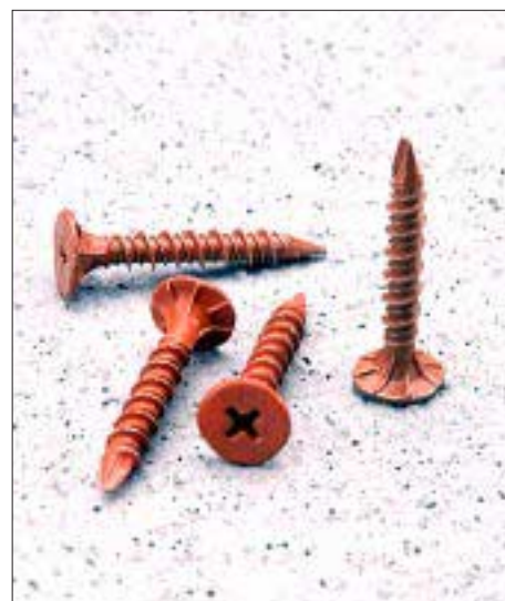
Figure 3. For fastening, use backerboard screws with a special anticorrosive coating that holds up better than zinc. A series of ridges on the underside of the head cut a countersink, so the oversize screw head draws up flush to the surface without pulling through.
