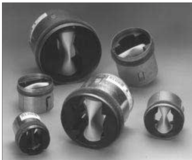
Figure 2. The Constant Airflow Regulator (CAR) installs inside standard round ductwork. As static air pressure increases, the silicone bulb inside the CAR automatically inflates, restricting the free area of the opening to maintain a constant measured airflow. CARs are available in a variety of standard sizes and capacities.
