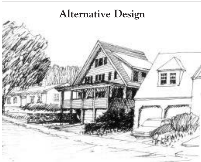
Figure 1. The author's alternative design narrows the existing building footprint and adds a south-facing deck at the first-floor level. A more practical entrance is created by cutting the grade down to street level and adding a stone retaining wall.
