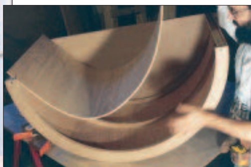
Figure 3. The author cut the curved frame and face trim for the vaulted top of the cabinet with a jig-piloted router (left), then skinned the assembled vault with bending plywood (above). The finished vault mounted easily into place with screws.
