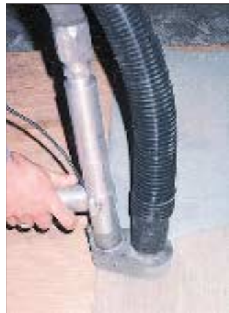
The Ecostrip paint-removing system produced virtually no contamination in tests sponsored by the Canadian government.
