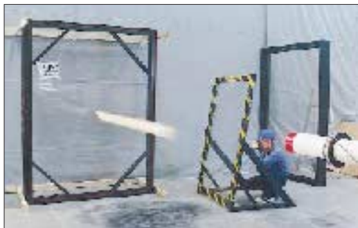
Windows and shutters approved by Dade County have to resist the impact of a 2x4 launched from a cannon.
