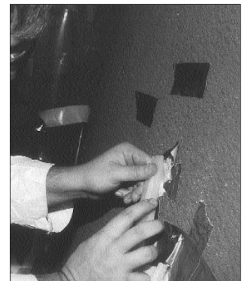
NASA maintenance crews deployed "Scare-Eye" balloons and repaired damage with duct tape after woodpeckers attacked the space shuttle's foam-insulated fuel tanks.
