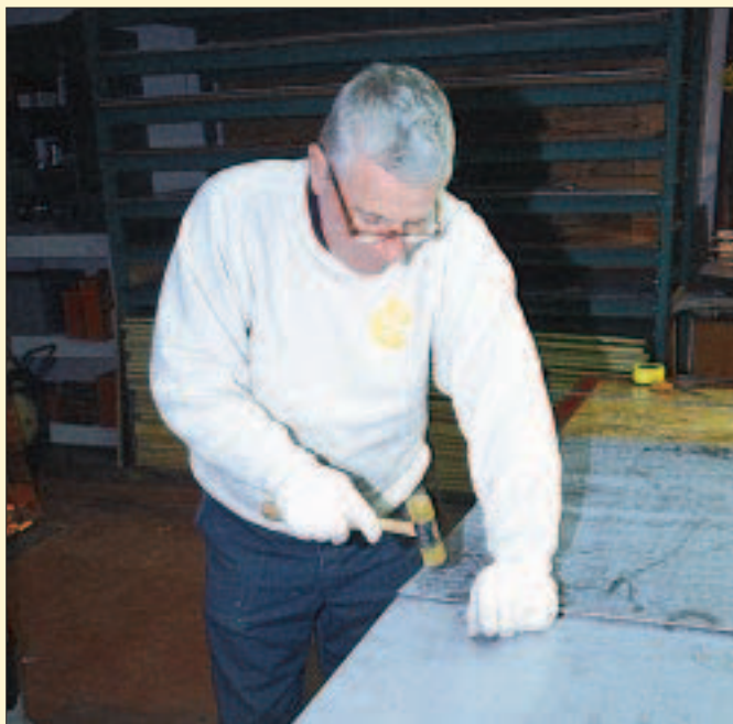
For extra strength, the author first joins large pieces of metal with a flat lock seam, then solders the joint (left). When soldering, heat the joint with the iron, then touch the solder to the heated metal (right).
