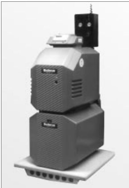
Figure 2. This combination boiler and domestic-hot-water heater features a preassembled pump/valve module (on top in black) and a built-in microprocessor that can be programmed for outdoor temperature reset, preset heating schedules, and boost after setback.
