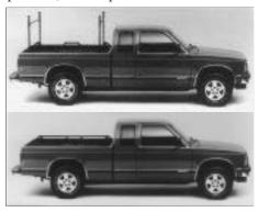
the ends. To take the rack down, remove the cross bars from the uprights (they come with a storage box that fits behind the seat), and fold down the upright rails. Assembly and disassembly each takes less than a minute.
