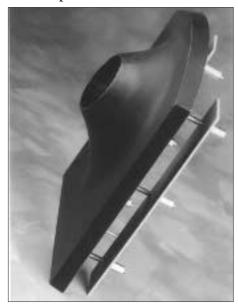
With the Kozy Kollar, you can flash vent-pipe penetrations without ever setting foot on the roof. The Kozy Kollar consists of a ¹/8-inch-thick steel frame, and a heavy rubber gasket and boot. Working from inside the attic, use the supplied template and a reciprocating saw to cut a hole in the
