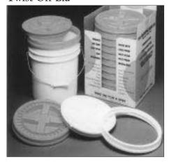
The problem with the lids on those 5-gallon paint and drywall pails is that you can't reseal them once they're removed. One solution is the two-piece *Gamma Seal*. The outer ring attaches to the lip of the pail and the inner lid screws to the ring to provide a locking, twist-off cover that's leakproof and airtight.
