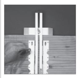
The company that makes *The Joister* claims it can cut the time it takes to install joist hangers in half, while increasing accuracy. The T-shaped Joister consists of a solid metal cross bar that slides up and down a channel in the center of a long vertical bar. To use it, mark the center of each joist on the header, and set the cross bar to the depth of the joist. With the cross bar
