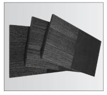
The shakes are designed for a 10-inch maximum exposure, weigh around 600 pounds per square (about midway between high-quality asphalt and slate), and come in three colors — Midnight (dark gray), Dusk (dark brown), and Sunset (light brown). The shakes are 22 inches long and 5, 7, or 12 inches wide. Starter pieces and hip and ridge cuts are also available.
