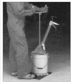
Buying high-viscosity caulk in five-gallon buckets and using a reloadable caulk gun can save a lot of money on some jobs, but reloading the gun is always a challenge. This new loader from Force-Flo will cut loading time in half for heavy materials like firestopping, trowel-grade caulk, and heavy mastics, according to the manufacturer. The advantage is in a new "split nut" design that more efficiently transfers
