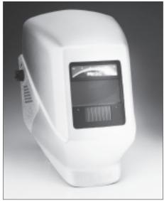
It may look like the hottest thing in virtual reality, but it's actually a new electronic quick-change welding helmet. The window goes dark automatically when it senses the spark of a welding rod. The sensitivity is adjustable for low-arc welding applications or high ambient light situations. The *Master* helmet features a switching speed of 1/25,000 of a second. It sells for \$360.
