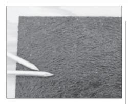
ment is a waterproofed fiberglass mat guaranteed to be dimensionally stable. The manufacturer claims it replaces both 15- and 30-lb. felt as an underlayment for asphalt shingles, metal roofing, and tile. The sample I examined looked like it would also provide excellent traction for workers on the roof. R-432 costs a bit more than plain old felt paper, but it's cheaper than having to replace wrinkled felt.
