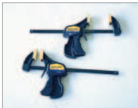
Figure 2. The author prefers Bessey bar clamps (left) for holding cabinets together. Quick-Grip Mini Bar Clamps (above) are useful where you must clamp one-handed. Because they lack the strength to lock the cabinets in place, however, the author uses them in combination with Bessey clamps.
