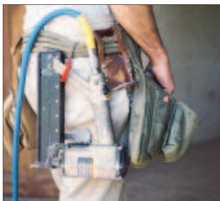
Figure 4. The handle from a drywall bucket makes a good belt hook for a finish nailer. Dipping the hook in a liquid plastic coating keeps it from scratching cabinet faces and other surfaces.
