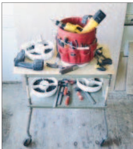
Figure 3. A rolling metal cart keeps supplies nearby during a kitchen installation. A Bucket Boss holds tools in a drywall bucket, while a set of round Drop-in-the-Bucket trays keeps fasteners neatly organized.
