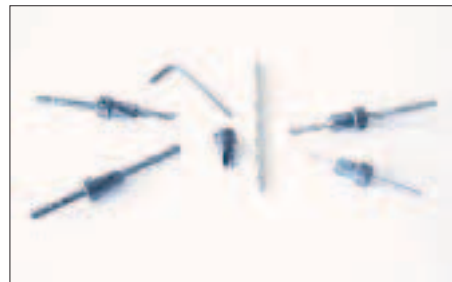
Figure 6. The author keeps several Fuller countersinks on the job, each set at the depth needed for a specific task. Switching between bits is much faster than repeatedly resetting the pilot depth.
