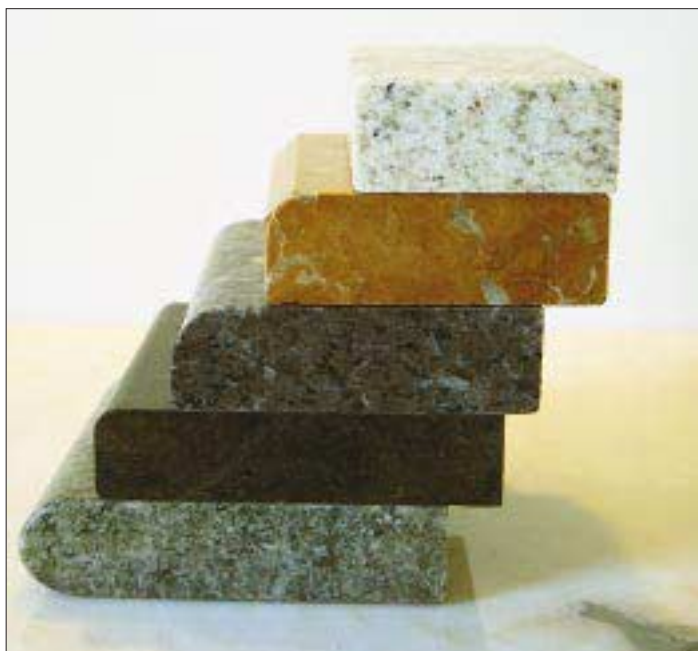
Figure 5. Edge treatments include (from the top down) flat eased, 1/4-inch x 1/4-inch bevel, half bullnose, pencil round, and full bullnose. Prices for edge treatments range from $14 to $34 per foot.
