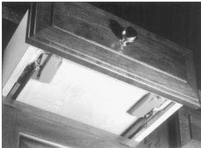
Figure 1. Standard, side-mounted drawer slides are inexpensive, but are unattractive on a traditionally styled cabinet. Invisible slides solve the problem by mounting beneath the drawer where they can't be seen.
