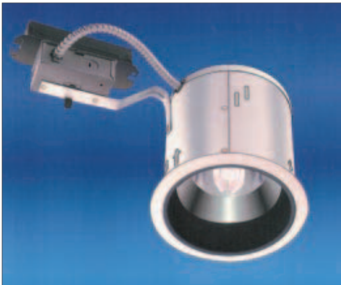
Figure 2. Compact fluorescent downlight bulbs are too tall to fit inside cans designed for incandescents. Instead, use cans made for compact fluorescents, like this one from Juno.
