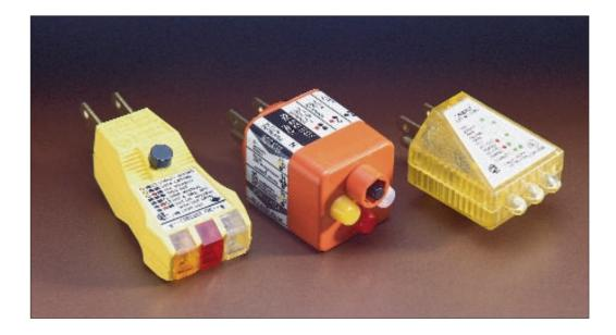
Plug-in testers are a safe, inexpensive way to troubleshoot 120-volt household circuits. By simply plugging in the tester, you get the results of a variety of tests, indicated by a series of three lights on the front of the unit. A key on the tester tells you what each particular combination of lights means.
