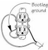
receptacle and turned on, this puts current on the grounding circuit in parallel with the neutral. That means anyone using an appliance anywhere on that branch would be in danger of shock.
