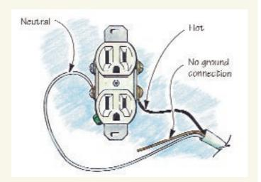
connection.) If the ground wire was cut, you should rewire the receptacle with a properly connected ground.
