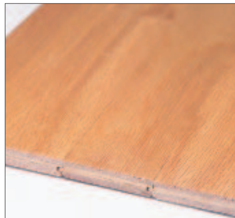
Figure 1. The \frac{1}{8} -inch-thick top veneer of this Robbins laminated floor is guaranteed for three sandings.
