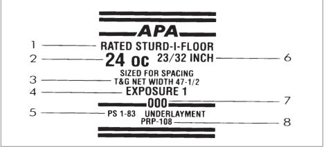
APA Sturd-I-Floor plywood panels are a combination subfloor and underlayment. The grade stamp (above) indicates the APA panel name (1), span rating (2), panel type (3 — in this case, tongue-and-groove), exposure classification (4), a number that corresponds to a general product standard (5), thickness (6), the number that describes the mill where the panel was made (7), and a number designating the APA performance standard that the panel is designed to meet (8).
