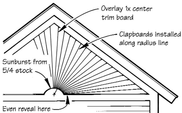
To fan wood clapboards, rip the butt edge of the clapboard to the appropriate taper, then lay this edge along the radius of a half circle. The clapboards should overlap each other at least one inch.
