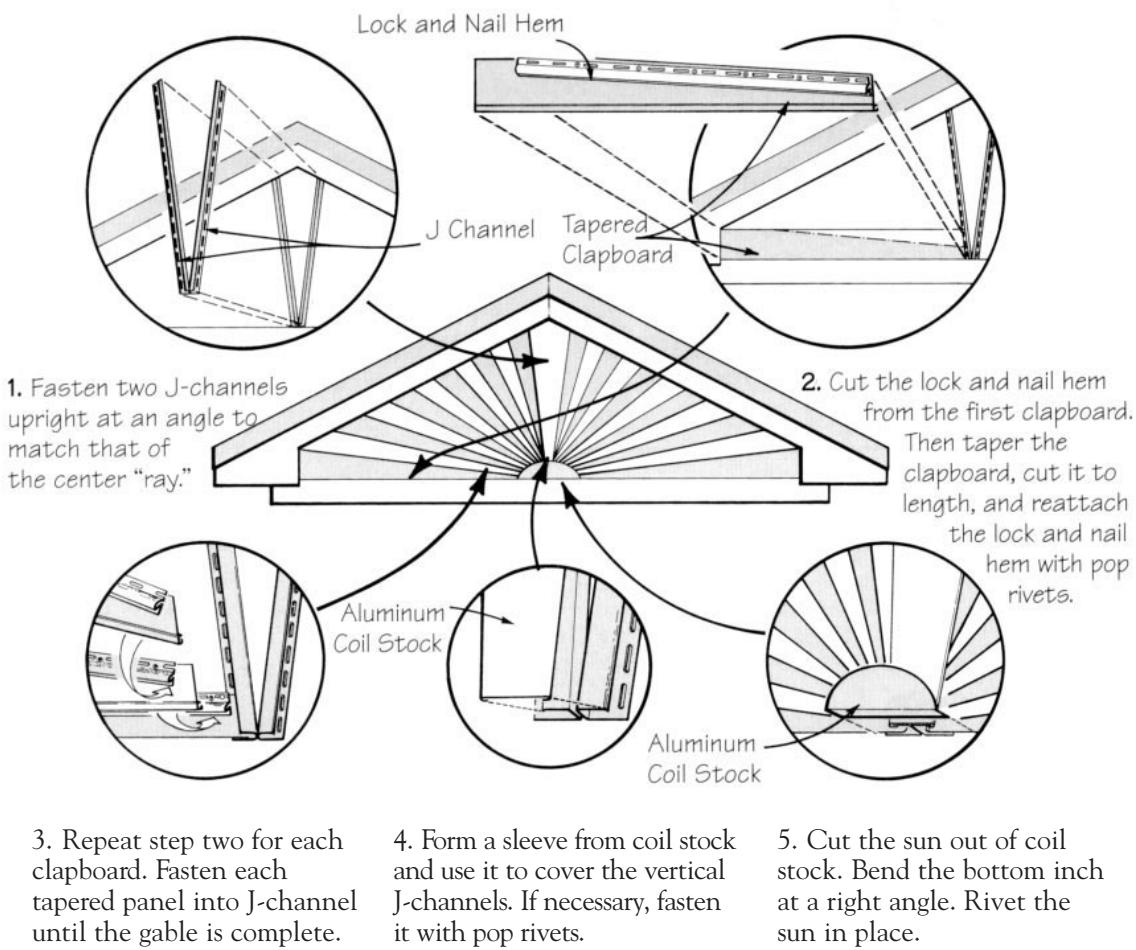
The sunburst is formed by fanning out vinyl panels on either side of vertical strips of J-channel, following the sequence shown.
