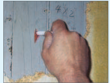
This test swab contains rhodizonate, a chemical that reacts with lead and turns pink if the paint contains around 0.5% or more lead by weight.
