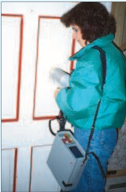
The author uses an XRF machine to test the paint on a door for lead paint. XRF gives instant results and will read through all layers of paint without marring the surface.
