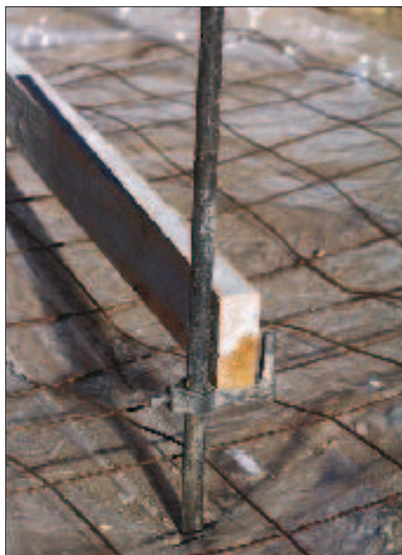
Figure 3. Steel stakes eliminate the need to cut wooden stakes for every job. These stakes are predrilled every 3 inches to accept fasteners and come with an optional screed hook.
