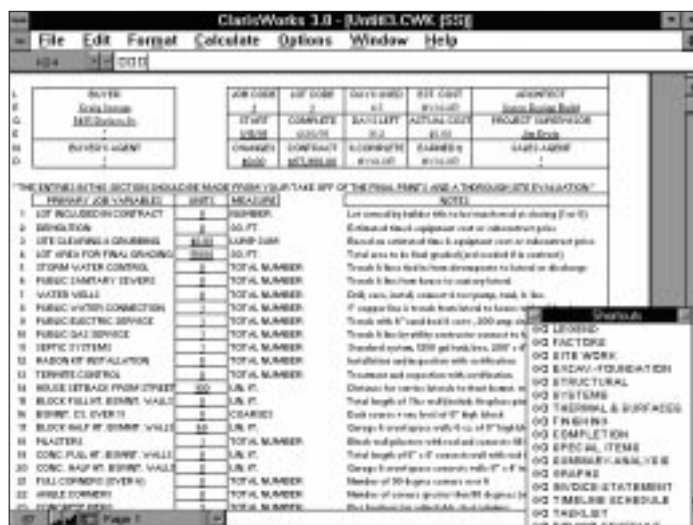
Figure 1. One of the first steps in building an estimate in GC Works is to enter values for each item in a list of Primary Job Variables that are used to calculate unit costs. Built-in macros make it easy to navigate to other parts of the spreadsheet by clicking on an item in the "Shortcuts" menu (lower right).
