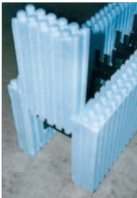
Figure 6. Grooves on the outer surface of a Greenblock form provide good surface bonding for finish coatings; dovetail grooves on the inner face accept end plugs. The knobs on top of each panel interlock into the bottom of the next course.
