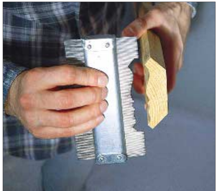
Figure 4. A profile gauge is useful for matching existing moldings that are no longer available. Include the cost of custom cutters — usually between $50 and $300 — to the trim estimate.
