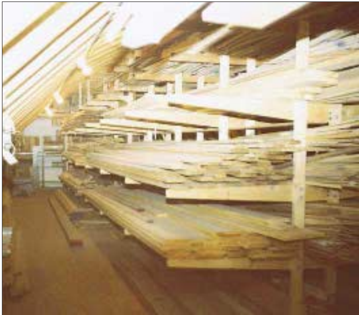
Figure 1. Millwork shops get their wood in random widths and lengths. It's important to provide a detailed list of finish sizes so the shop can pick boards that minimize waste.
