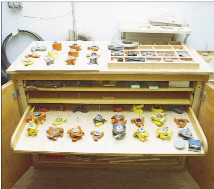
Figure 3. Many small shops have a selection of cutters that lets them crank out stock molding profiles on short notice. Often the shop can use several cutters in combination to match an unusual profile.
