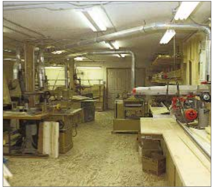
Figure 6. Adequate lighting is critical for doing safe, precision woodworking. This shop has plenty of general lighting as well as task lighting for specific machines.
