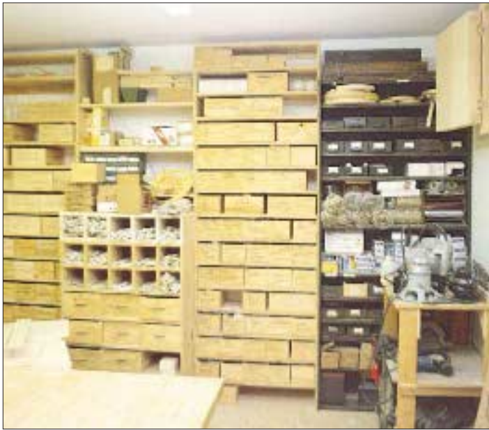
Figure 5. Good organization is a clue to a shop's professionalism and ability to meet deadlines. This shop uses a wall of drawers to systematically organize small pieces of hardware.
