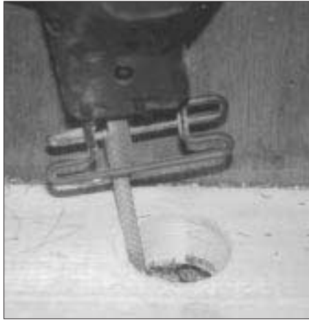
Bosch includes a rasp among the many accessories available for the In-Line Jigsaw. Here it is used to widen the hole in a wall plate for a plumbing line.
