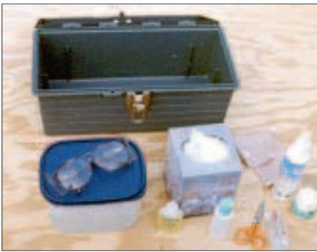
*The author's crew keeps their safety glasses clean and free of scratches using this simple cleaning station. It contains a rinsing basin, defogging solution, and soft tissues, plus items such as a glasses repair kit and nail polish remover for removing paint splatters from plastic lenses.*
