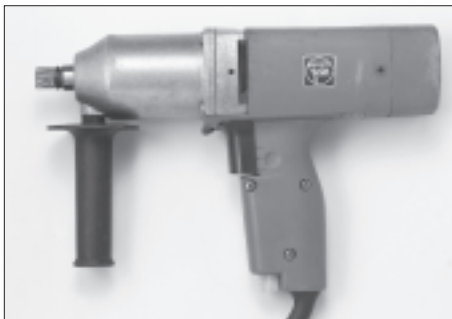
A quick turn of the black housing cap on the Porter-Cable 625 (top) reverses the motor direction. The Fein ASbe 642 (above) is the only electric impact wrench on the market with variable speed and variable torque.
