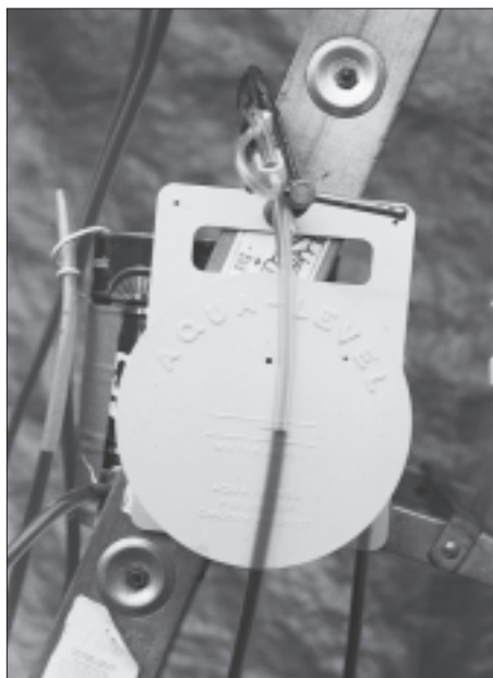
The author clamps this Aqua-Level to a ladder, then takes the "working end" (shown on clamp handle) to mark out a level line.
