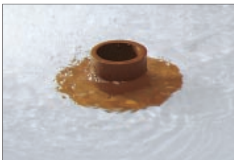
Figure 9. The Tub Stopper lets you test a shower pan for leaks without worrying about a flood — the hole in the center allows for overflow.
