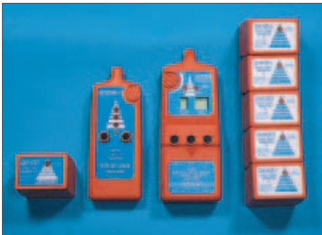
Figure 6. The Circuit Pup Breaker Finder helps you figure out which breaker controls which outlet. A transmitter plugs into an outlet, and a receiver traces the signal anywhere along the branch back to the panel. The device can be used on live or dead circuits.
