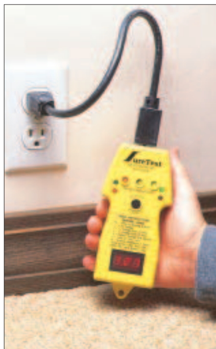
Figure 5. The SureTest Branch Circuit Analyzer checks for proper circuit polarity, as well as determining the quality of a ground connection. It can locate false grounds, where the neutral and ground wires are shorted, and will measure the voltage drop at any outlet.
