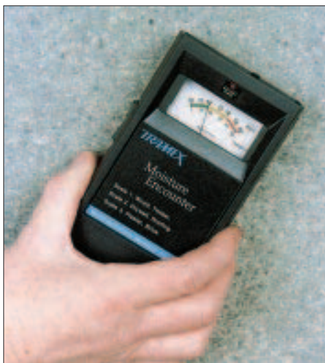
Figure 3. The Tramex Moisture Encounter costs $300, but can pay for itself the first time it finds a hidden plumbing leak. Because the sensors are wrapped in rubber pads, they won't mar finish surfaces.
