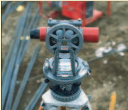
Figure A. A transit scope can rotate 360 degrees around a vertical axis and nearly 60 degrees up and down. When all of the bubble vials read level, a scope locked into position at zero degrees elevation will describe a level line no matter which direction it is pointing.
