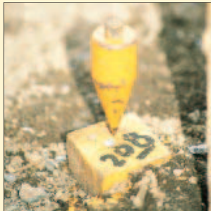
Figure B. The plumb bob, or plummet, attaches to the exact center of the transit frame. It can be used to set up the transit directly over a point or line.
