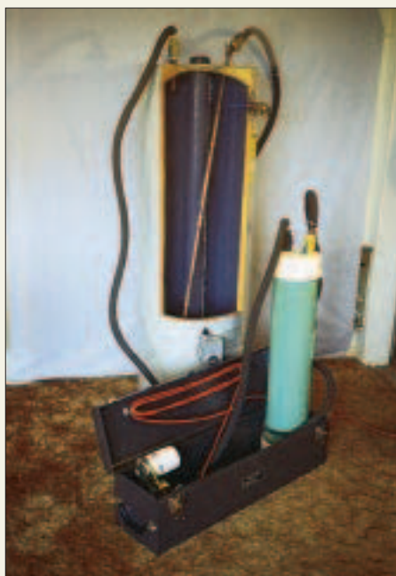
Figure C. The author designed the Muck-Vac to pull sediment off the bottom of the tank, filter it, and return clean water through the dip tube.
