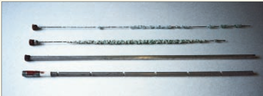
Figure B. The slow corrosion of a magnesium or aluminum anode rod protects glass-lined tanks from rust. Check the anode every few years and replace it if 6 inches or more of the steel core wire is exposed or if the rod is coated over with a brittle scale. Use a flexible-link rod where overhead clearance is restricted.
