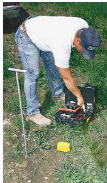
Figure 3. The author sets up a seismograph to record the force of the blast.
