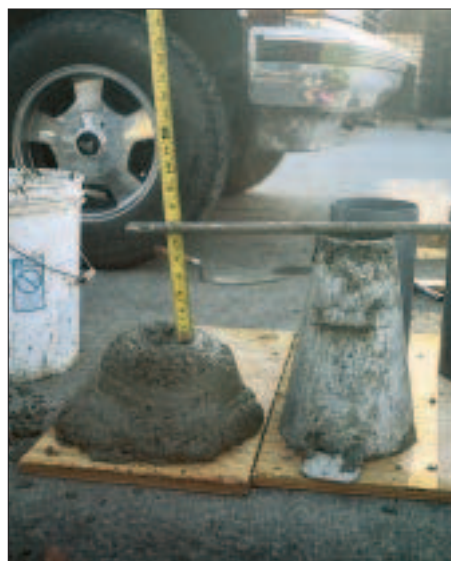
Figure 2. The best way to guarantee concrete slump at the site is to perform a cone slump test (left). The wetter the concrete, the higher the slump (right).
