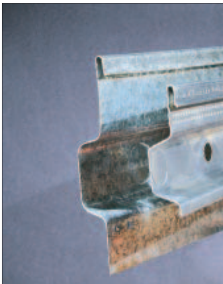
Figure 9. These galvanized steel forming materials create a "keyed" control joint — essentially a tongue-and-groove — that helps keep adjacent slab sections in a flat, horizontal plane.
