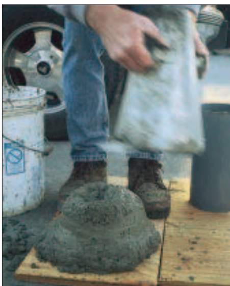
Figure 2. The best way to guarantee concrete slump at the site is to perform a cone slump test (left). The wetter the concrete, the higher the slump (right).
