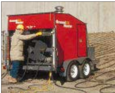
The oil-fired Ground Heater (left) applies heat directly to the earth through rubber tubing, thawing out a foot of frost per day. For deep frost, 3-foot heating probes are inserted into drilled holes (above).
