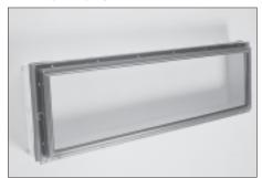
Retrofitting skylights is complicated when existing framing is in the way. Sweet 16 roof windows fit into a rough opening just 14½ inches wide, so you don't have to cut any rafters or install any headers. The fixed roof windows come in two sizes: 46½ inches long and 57 inches long. Options include low-e glass and argon-filled panes. The smaller window costs about \$200 and the larger one costs around \$210. Both prices include a step flashing kit for installation.
