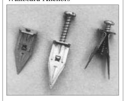
Here's a wallboard anchor that does a little less damage to the wall than some others on the market. The Legs anchor has a thin profile in the closed position that can be tapped into the wall (without a pilot hole) with a hammer — even with the end of a screwdriver. Driving the screw in spreads the legs and secures the anchor. They're rated to hold up to
