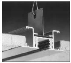
${f T}$ rack lighting added onto a suspended ceiling grid usually looks like it was cobbled together. The new Capri Integral Track replaces one runner in the grid, so the track is recessed above the ceiling. The track can be wired as two separate circuits that can be dimmed independently since each has its own neutral wire. Connectors for turns and junctions are also available.
