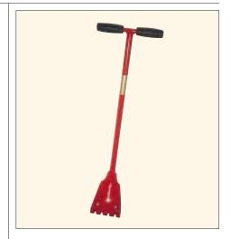
up. It's about 30 inches long and has a 5-inch-wide hardened steel blade with four notches that help the angled tip slip under nails and pop them free. The padded T-handle grip makes it easy to operate the stripper with two hands. The Tear-off Tool is welded out of plate and tubular steel and sells for around \$25.
