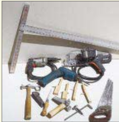
Hanging tools (clockwise from right): Drywall handsaw, hole compass, edge-ripping stripper, keyhole saw, Surform plane, drywall hatchet, 4-foot T-square, electric and battery-powered screw guns.
