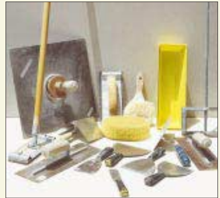
Finishing tools (clockwise from upper right): Paddle mixer, assorted knives and trowels, pole sander, hawk, hand sander, sponge, brush, mud tray.
