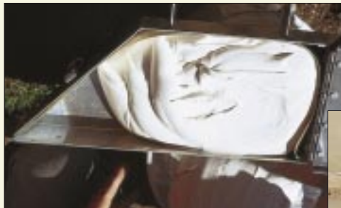
A taping banjo makes quick work of bedding drywall tape. You fill the mud compartment (above), and the tape is coated with compound as it's pulled from the banjo (right).
