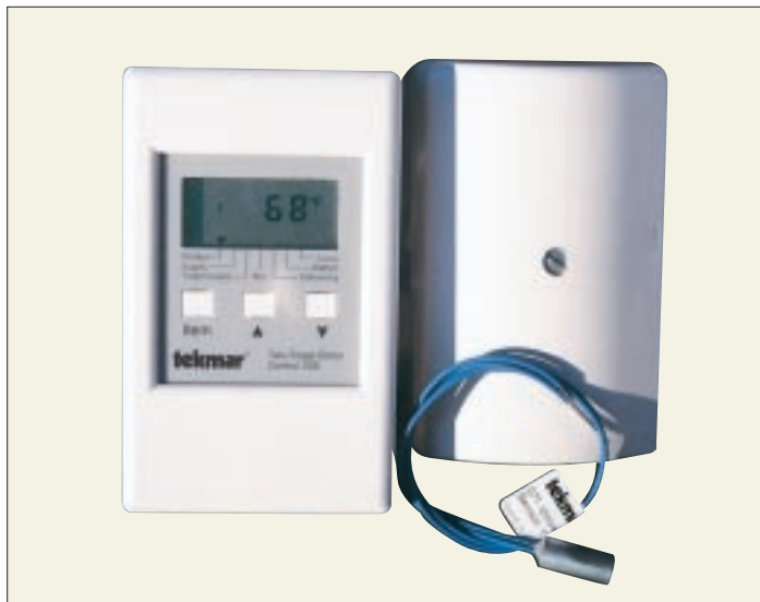
Figure 3. Weather-responsive boiler controls like this one from Tekmar adjust the temperature of boiler water to match changes in outdoor temperature. This increases system efficiency because the boiler never heats the water more than is necessary to keep the house at the desired temperature.
