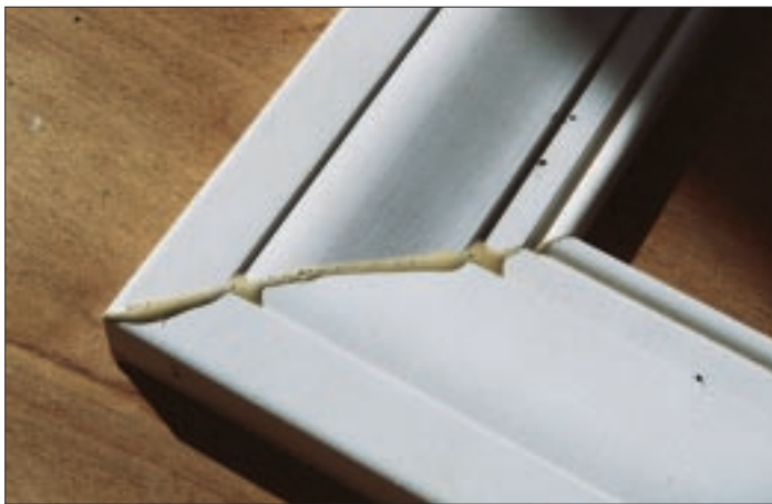
Polyurethane glues foam and expand as they set, helping to fill gaps in the joints (left). The squeeze-out can be cleaned immediately with mineral spirits, but the author prefers to use a chisel on the excess after it has dried (right).
