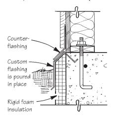
in a slab addition with the poured-inplace flashing shown above. The top flange ties into the concrete, where it's easy to visually inspect for a "termiteproof" seal. I placed the foam right into the form before pouring and in some places even used the foam-and-flashing as my form. I'm sure this flashing detail would adapt just fine to stem walls, too.
